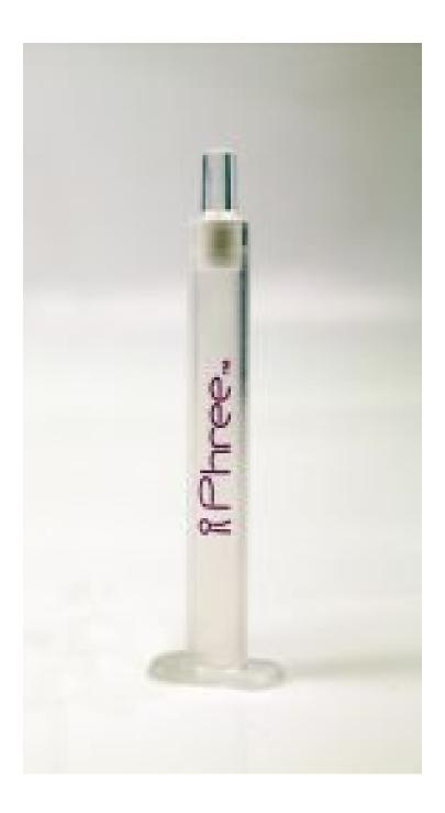
First offered in 96-well plates for automated applications, the Phree sorbent in 1 mL tubes is ideal for users with lower throughput needs as well as for labs who do not have the ability to automate. Phree delivers fast cleanup of plasma samples in pharmaceutical and clinical research laboratories.
