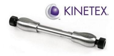
Phenomenex has added an advanced line of HPLC columns to its core-shell line, the Kinetex EVO C18. These columns are said to be made of a patented organo-silica grafting process that utilizes uniform stabilizing ethane cross-linking to create a unique selectivity and ultimately, pH stability from 1-12.
