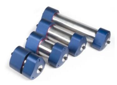
The new 30 mm column will enable increased loading of sample and throughput. With the addition of this larger diameter column, Phenomenex offers core-shell media line can be used from analytical scale through scale-up to purification.
