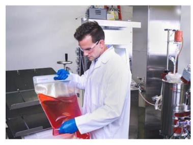
US-based Thermo Fisher Scientific Inc. is contributing to the sustainability of biologics therapy manufacturing by leveraging plant-based materials, rather than fossil fuel materials, to deliver lower-carbon, biobased films for its single-use technology bioprocessing containers (BPCs).
