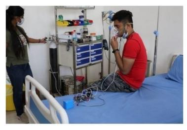
The Indian Institute of Technology (IIT), Ropar has developed a first-of-its-kind oxygen rationing device – AMLEX that supplies a required volume of oxygen to the patient during inhalation and trips when the patient exhales CO2. This process saves oxygen which otherwise unnecessarily get wasted.
