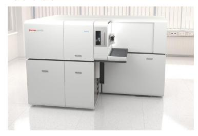
A new inductively coupled plasma mass spectrometry (ICP-MS) instrument has been designed to enable scientists working in earth sciences, nuclear safeguards and biomedical research to conduct reliable, high-precision isotope ratio analysis across a wide range of applications, without compromising sensitivity, stability or ease-of-use.
