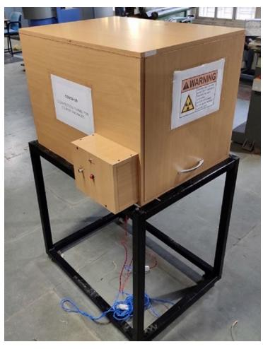
Researchers at the Indian Institute of Technology Mandi have developed an Ultraviolet-C (UV-C) light-based portable disinfection box at a cost of ?35,000 to disinfect metallic, plastic and cardboard products like wallets, keys, spectacles, bags, courier packages and parcels, among others, to minimise the risk of COVID-19. Minimising the risk is the key because this virus can live on these surfaces for up to 3 days.
