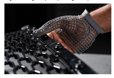
Engineers from Jaguar Land Rover are working on the next generation of protective workplace clothing – a lightweight 3D-printed glove which could help better protect employees from the threat of a musculoskeletal disorder.
