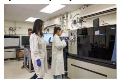
Researchers can now apply a range of ion beam species within one focused ion beam (FIB) scanning electron microscopy (SEM) instrument with the new Thermo Scientific Helios Hydra DualBeam system.
