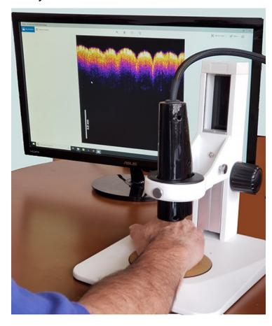
Using sound vibrations and pulses of near-infrared light, a Rutgers University scientist has developed a new "virtual biopsy" device that can quickly determine a skin lesion's depth and potential malignancy without using a scalpel.
