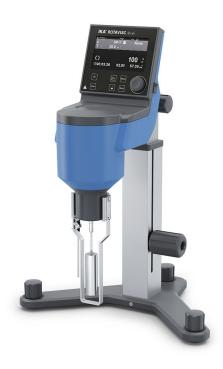
After it's been produced, stirred and shaken, the viscosity of a sample can now be measured with the new ROTAVISC series from IKA. This parameter indicates the fluidity of a substance and is important for quality control in all manufacturing processes and even early on in the application in the research laboratory. ROTAVISC is the most functional viscometer in its class.
