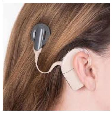
A cochlear implant is an electronic device that takes over the work of the human ear in converting sounds to electrical signals that the brain understands as sounds and delivers them to the brain via the hearing nerve, after fine tuning the sound much like the graphic equaliser on a music system, via an electrode array surgically implanted into the inner ear.
