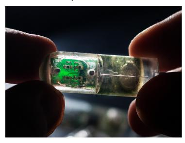
A team of researchers from the Massachusetts Institute of Technology (MIT) in the US has developed an ingestible sensor that features genetically engineered bacteria to diagnose bleeding in the stomach or other gastrointestinal (GI) problems.
