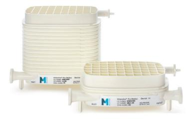
Merck, a leading science and technology company, has introduced Viresolve® Barrier capsule filters to reduce the risk of bioreactor contamination.
