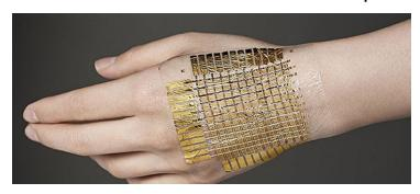
A team of scientists at the University of Colorado, US has developed a new type of malleable, self-healing and fully recyclable electronic skin that has applications ranging from robotics and prosthetic development to better biomedical devices.
